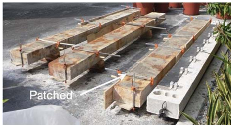
Figure 4.17 - Concrete patching chipped areas (B1 to B3)
