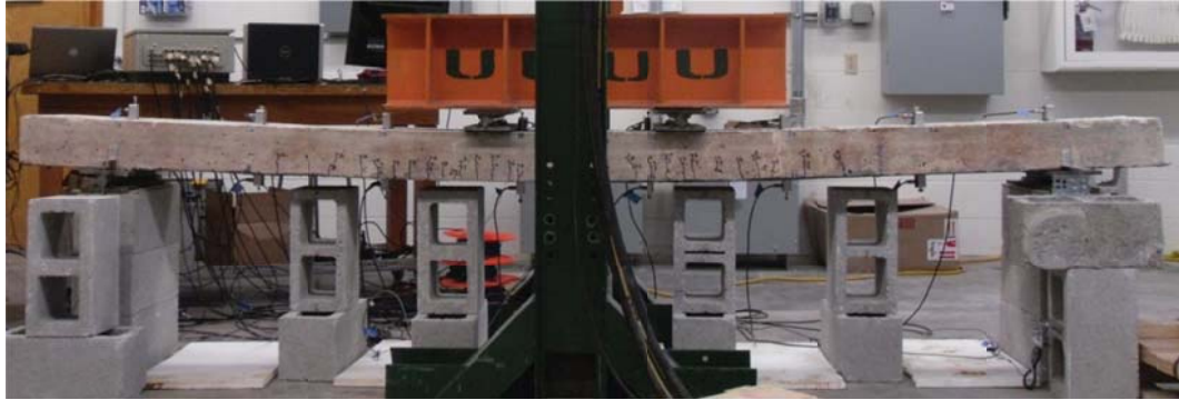
Figure 4.24 - Test setup with bended specimen close to failure
