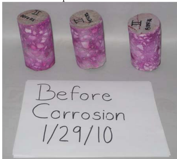
Figure III.D.2 - Core evaluation of concrete carbonation before corrosion
